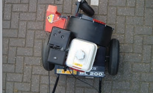
Fanhouse is mounted slightly in offset for efficient working
