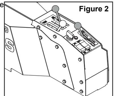
To start the engine from cold pull the throttle lever back to the choke position (See **Figure 2**), and turn the ignition key. Release the key once the engine has started and allow the engine to warm up. To stop the engine turn the ignition switch to the off position. Use the recoil start if the battery is not charged sufficiently to start the engine.
