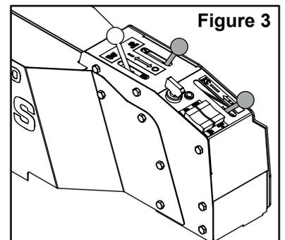
The **Brush-Pro** is driven by a Hydrostatic Axle, with the axle engaged (lever fully out) pressing the top of the pedal gives forward motion and pressing the bottom of the pedal puts the **Brush-Pro** into reverse. Releasing the pedal stops the **Brush-Pro**. The drive is proportional to the travel of the pedal.
