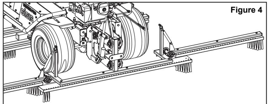
To engage the oscillating motion pull the centre brush drive lever back to the on position, (See **Figure 5**). Both the mechanisms that control the brushes compensate for ground clearance allowing them to be fully lowered onto the ground. The engine will cutout if the centre brush drive is engaged with the brake lever in the on position, thus protecting the centre brush oscillating mechanism.
